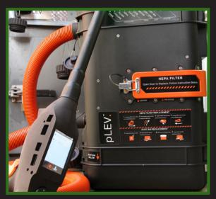
The pLEV™ system works by creating negative pressure-controlled environments in electrical cabinets. Dust is disturbed using the pLEV™ SmartLance and extracted safely and effectively using the pLEV™ Extractor.
